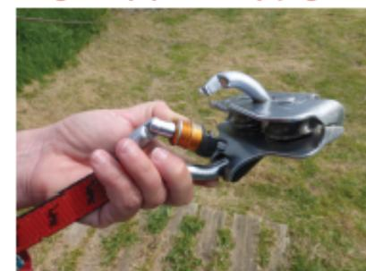
Two dynamic safety ropes with a hook and a semi-automatic karabiner and a red colour code One static safety rope with a pulley and a semi-automatic karabiner. To open this carabiner, drop down the orange ring and then push in with your finger
