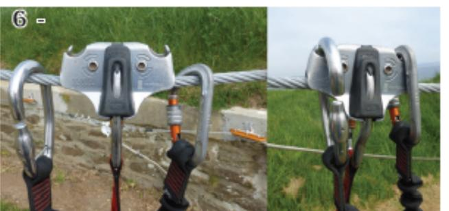
Put the pulley on the cable in front of your hook and add your Sit completely down in your harness... If ever you karabiner in front of the pulley. Check whether the pulleys rolls don't get to the end... well on the cable then put the karabiner and the hook on top of the pulley.
