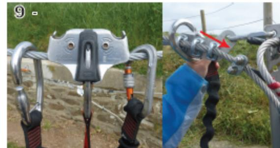
At the end of the zip wire, lift the karabiner and the hook off the pulley and put them on the cable.
